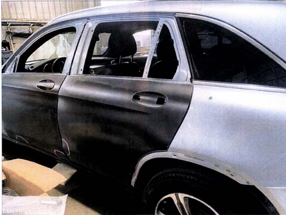
new doors -- trial fit
