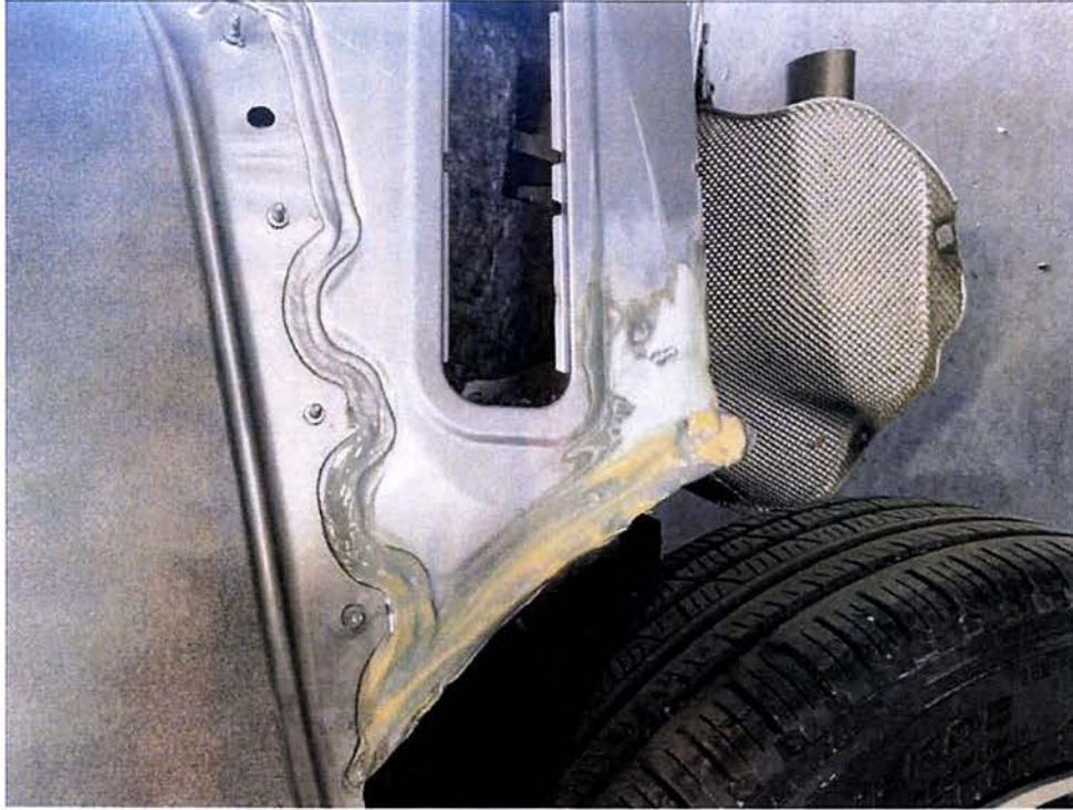
lower qtr repairs
