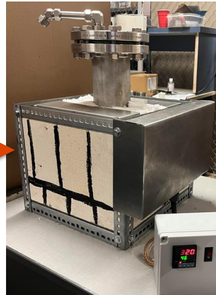
Plastic is directly loaded into reactor and heated to 460°C
