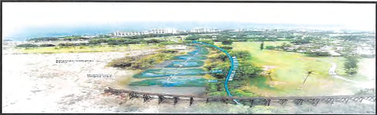
Figure 26. Detention Basins in Series
