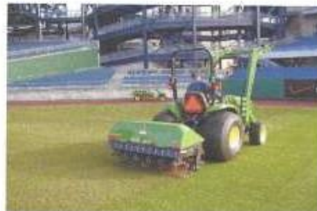
9. Core aerator (hollow tine cultivation) used on athletic fields (photo: L. Wood)
