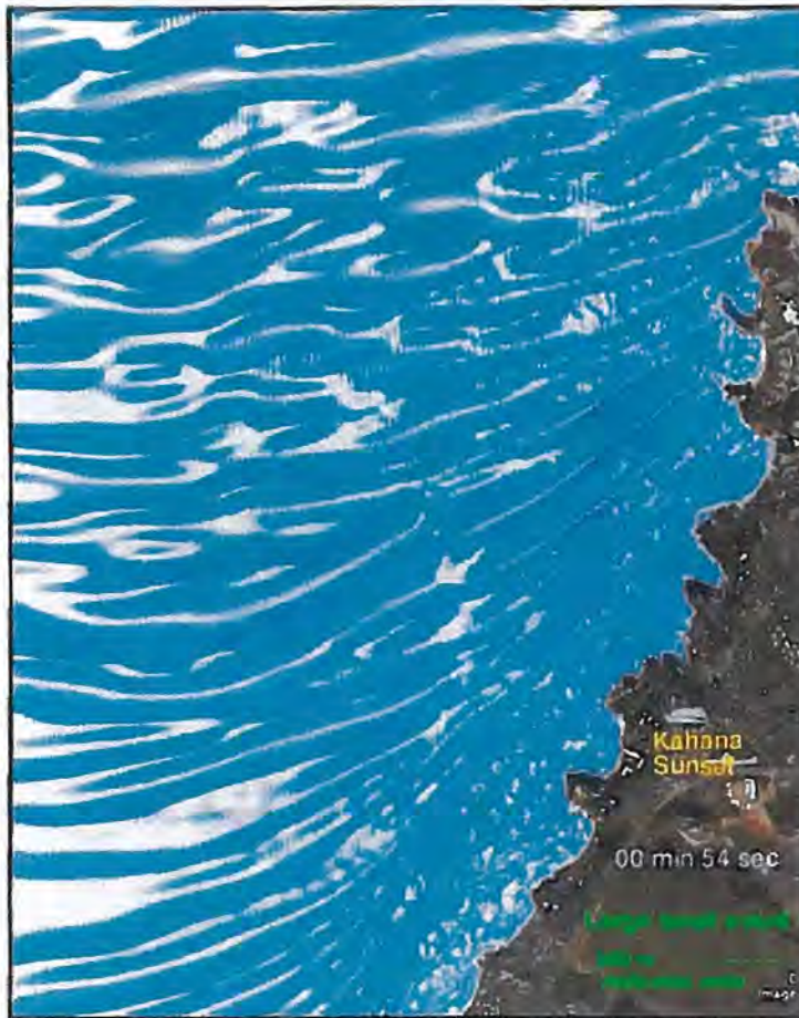
Figure 8- Wave Transformation at Northwest Maui for the Peak Swell Event
