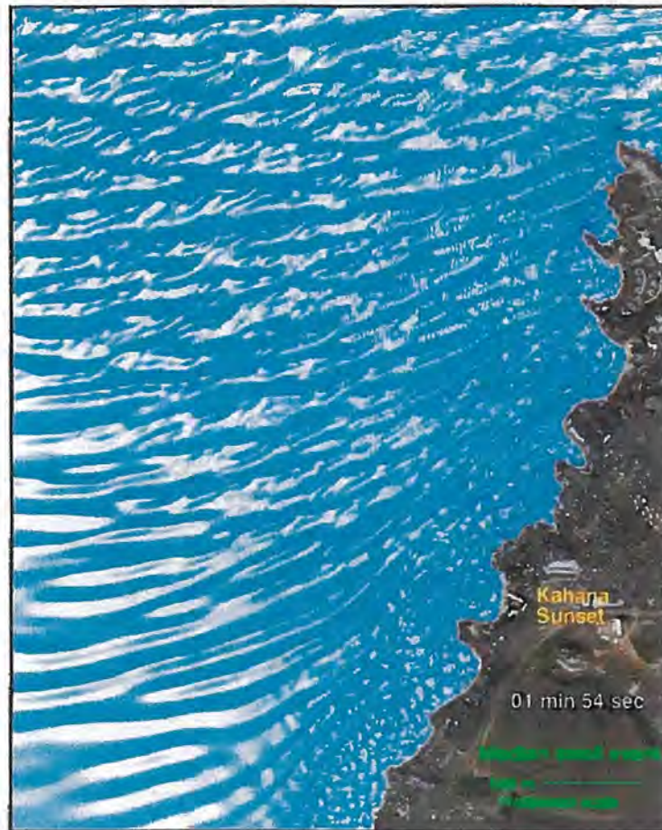
Figure 15- Wave Transformation at Northwest Maui for the Moderate Swell Event
