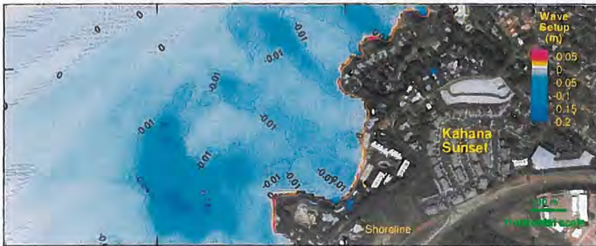
Figure 18- Wave Set up for the Moderate Swell Event.
