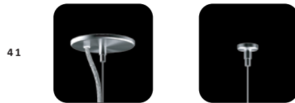
4" diameter machined power feed and 1-1/4" diameter machined non-power feed canopy. Offers minimal ceiling treatment while maintaining the ability to cover mistakes. Requires a 1/4-20 stud securely fastened to the ceiling. Mill, anodized, and powder coat finishes available.
