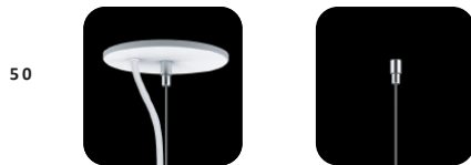
5" diameter power feed canopy and no canopy on the non-power feed side. Minimal aesthetic. Requires a 1/4-20 stud securely attached to ceiling. Works well with continuous runs where the power can be carried inside the fixture.
