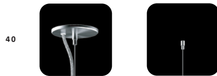
4" diameter machined power feed canopy and no canopy on the non-power feed side. Minimal aesthetic. Requires a 1/4-20 stud securely attached to the ceiling. Works well with continuous runs where the power can be carried inside the fixture. Mill, anodized, and powder coat finishes available.
