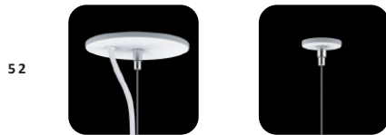
5" diameter power feed and 2" diameter non-power feed canopy. Offers a more minimal ceiling treatment while maintaining the ability to cover up mistakes. Requires a 1/4-20 stud securely fastened to the ceiling.
