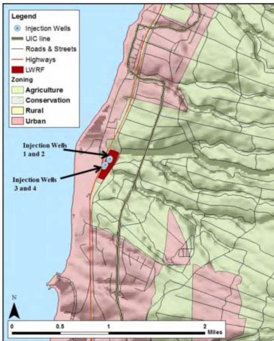
Figure 1-3: Location of the LWRF in relation to the coast and the UIC line. LWRF Injection Wells 1 and 2, which receive the majority of treated wastewater effluent, lie to the northeast of Wells 3 and 4.
