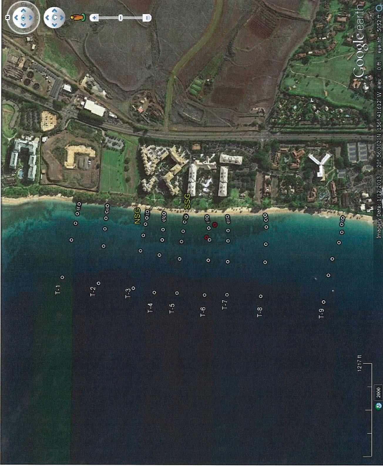
EXHIBIT 2. Satellite image of Kahekili Beach and offshore reef showing locations of nine water sampling transects. Water samples were collected at the ocean surface, mid-way through the water column, and just above the sea floor at eight locations along each transect (white circles). Locations of the North and South seep groups (NSG, SSG) are also shown as yellow circles. CRAMP monitoring stations are shown as red circles.
