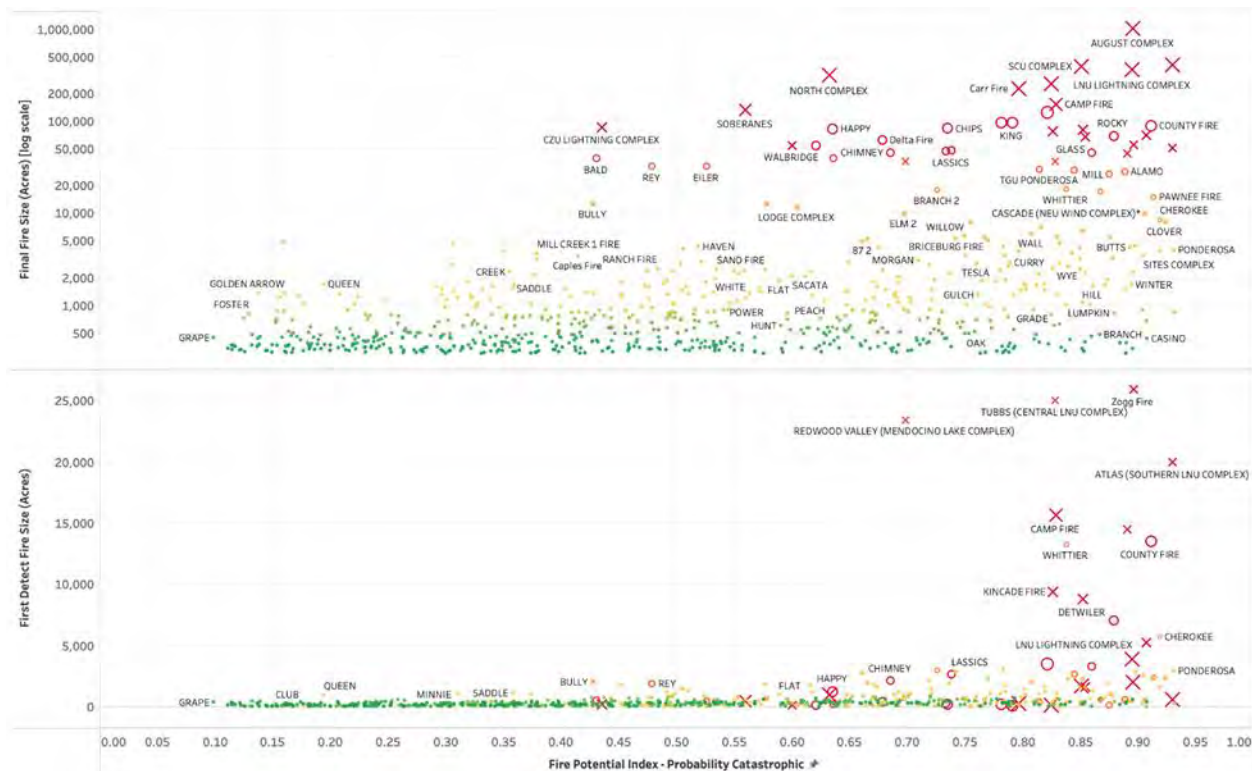
FIGURE PG&E-4.5.1-16: FPI P(CATASTROPHIC) ONLY FOR FIRES VS THE FINAL FIRE SIZE (TOP) AND THE FIRE SIZE AT FIRST SATELLITE FIRE DETECT ONLY (BOTTOM)
