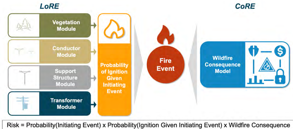
FIGURE PG&E-4.5.1-3: 2022 WDRM V3 COMPOSITE MODEL ARCHITECTURE
