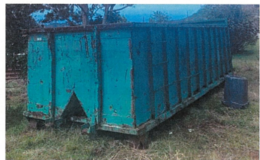
Figure 12. Roll-off dumpster for debris removal
