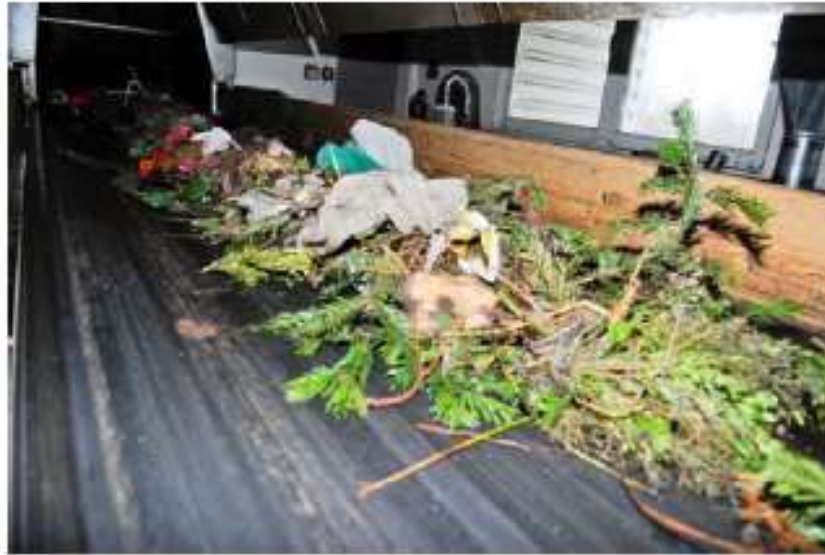
Extracting Metal, Plastic Bags or other Contaminants
