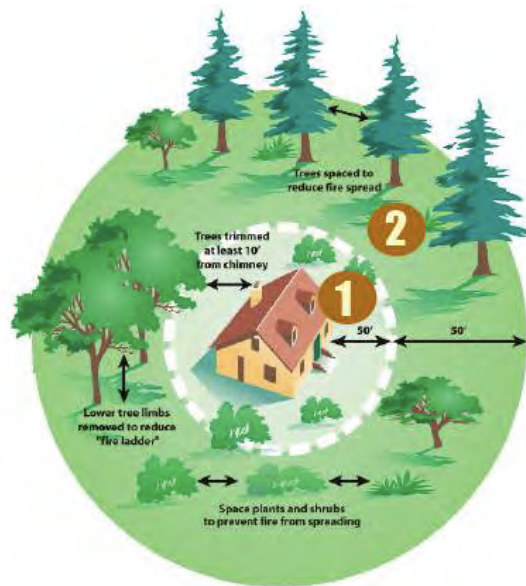
Figure 9. Defensible space zones around structures. 28
