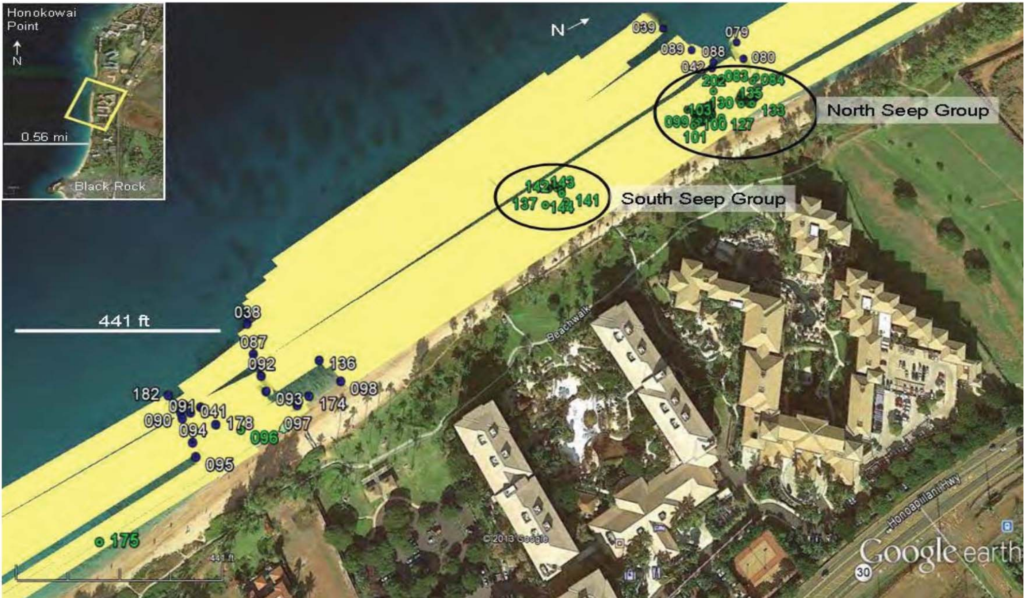
EXHIBIT 46. Area covered across Kahekili Reef during submarine spring survey during Groundwater Tracer Study. The area surveyed is shown in the yellow box of the map insert. Blue dots with white numbers represent the start and end of the transects; the transect widths (in yellow) are directly proportional to the visibility of the scuba divers at the time of the survey. Green dots with numbers represent samples collected from submarine springs, with the exception of 096 and 175, which were from diffuse discharge (Appendix Table A-6 of the Groundwater Tracer Study).
