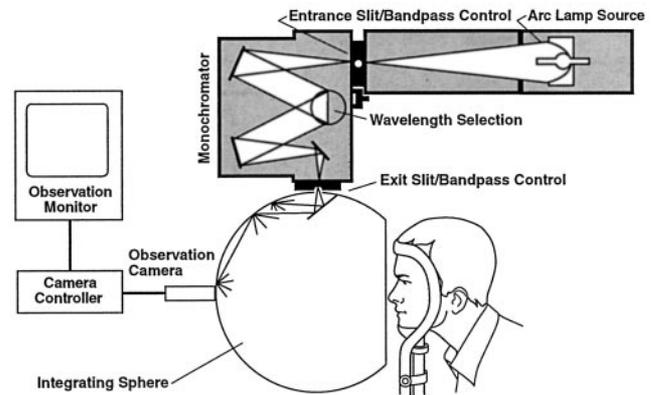
**Figure 1.** This diagram illustrates the experimental electronic, optic, and Ganzfeld dome exposure array. This apparatus provides a uniform, patternless stimulus that encompasses the subject's entire visual field. For clarity, the subject's head is shown slightly withdrawn from the opening of the Ganzfeld dome. During all light exposures, the subjects' bony orbits are completely enclosed in the dome walls, providing complete exposure of their visual fields.
