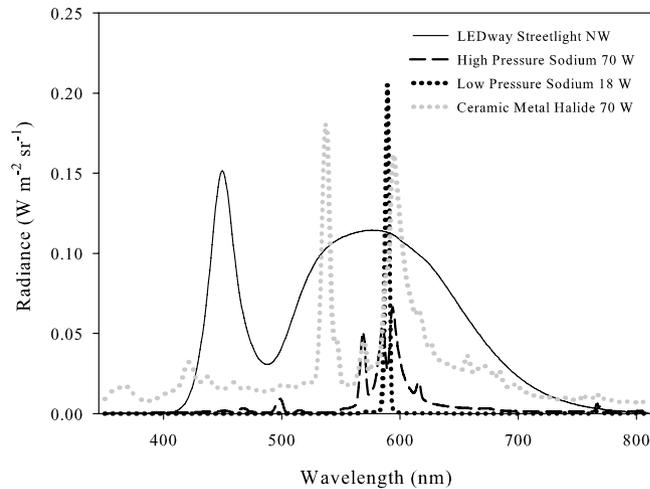
**Figure 1.** Spectra of different artificial light sources in use: LEDway - white LED (solid black line), high pressure sodium (dashed black line), low pressure sodium (black dotted line), and ceramic metal halide (gray dotted line). The spectra were obtained from [http://ngdc.noaa.gov/eog/night\\_sat/spectra.html](http://ngdc.noaa.gov/eog/night_sat/spectra.html).
