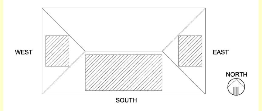
Plumbing vents and other roof penetrations to avoid center 3/4 of roof area on South, East and West faces.
