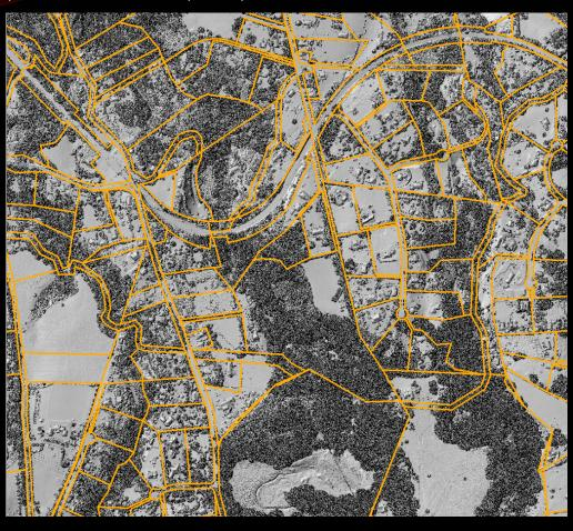
BARE EARTH LIDAR, SHOWING THE GROUND BENEATH VEGETATION, A RIVER BED AND OTHER GROUND ANOMALIES IN THE KAUPAKALUA AREA WITH TAX PARCELS
