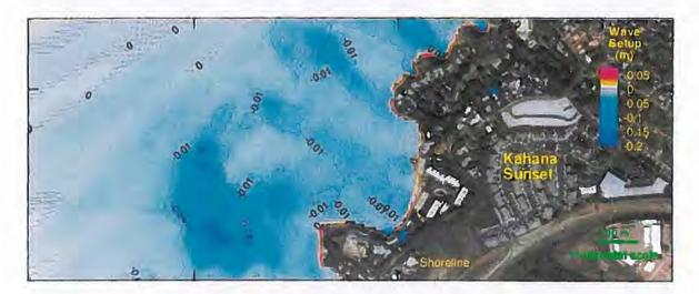
Figure 18- Wave Set up for the Moderate Swell Event.
