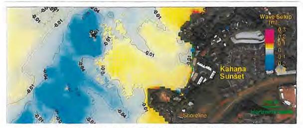
Figure 11- Wave Set Up for the Peak Swell Event
