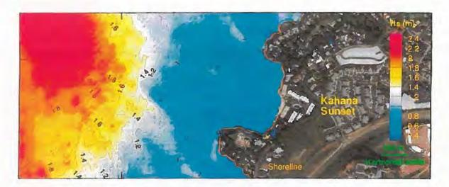
Figure 9- Significant Wave Height for the Peak Swell Event
