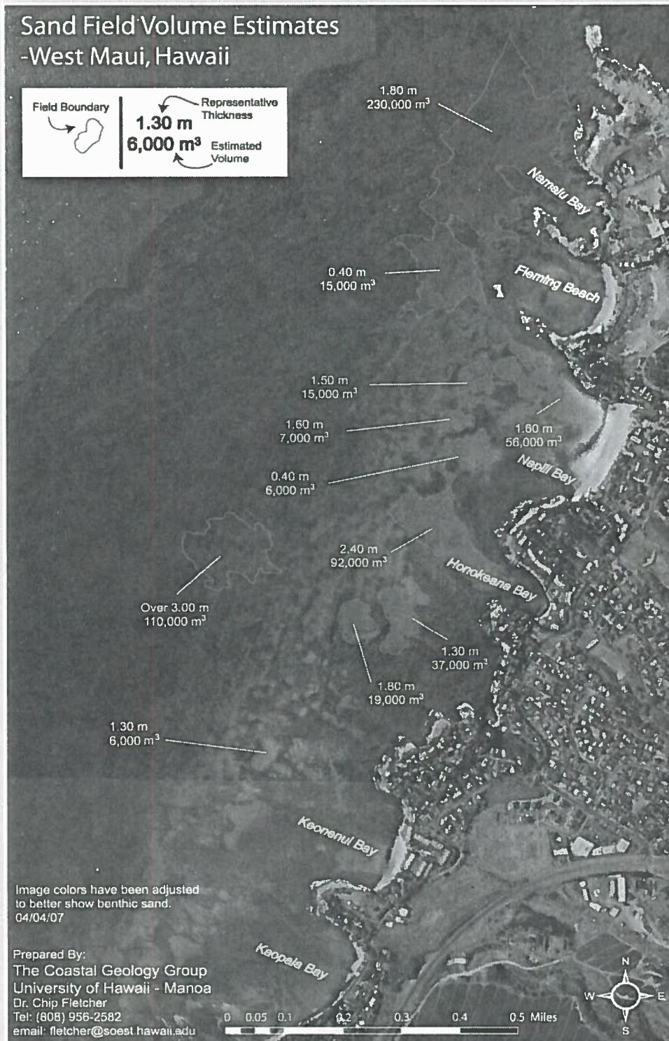
Figure 12. Offshore sand resource inventory for potential beach nourishment sand source, conducted by the University of Hawaii for the Napili Bay and Beach Foundation. (Image: University of Hawaii Coastal Geology Group)
