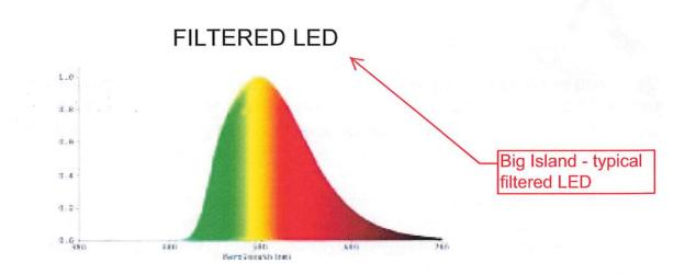
Spectrum Parameters Blue content (400nm-700nm): 0.14%Peak wavelength: 579nm
